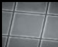
With a pixel gap of only 0.45µm, a smooth picture with no visible grid is obtained.
